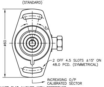
SHAFT FLAT ALIGNED WITH REFERENCE
